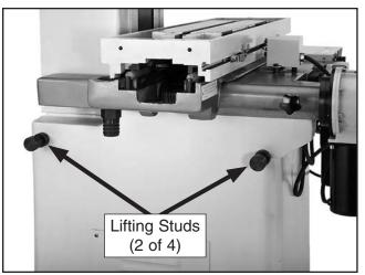
Figure 13. Lifting studs (2 of 4 shown).
